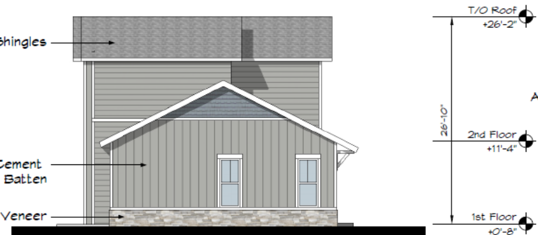
SIDE ELEVATION - PH3 DUPLEX
