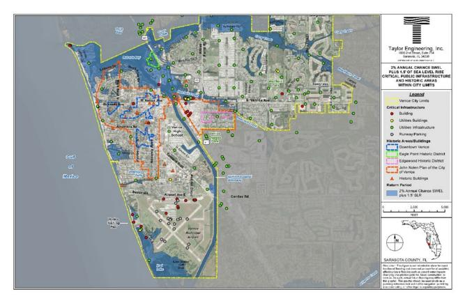
Figure 3.1 Venice Island Inundation Map under the 2% SWEL plus 1.5 FT SLR Scenario
