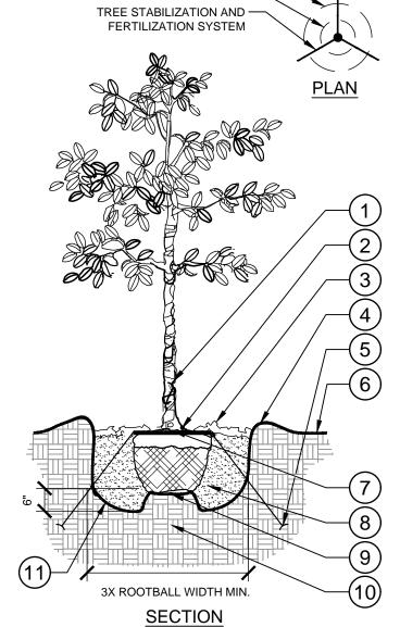
(2) 6" DIA. CLEAR OF MULCH AT TRUNK FLARE. 3 ) 3" MINIMUM MULCH AS SPECIFIED. WHERE TREES ARE PLACED IN SOD, MULCH RING FOR TREES SHALL BE 6' DIAMETER (MIN.) OR AS DIRECTED BY OWNER'S REPRESENTATIVE
