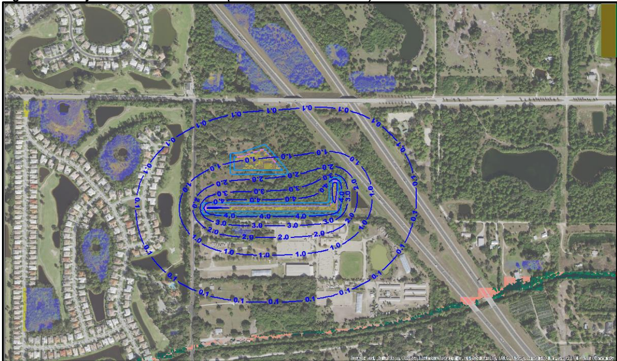
Figure 3. 42-day construction of Pond 1 (dewater to elevation 3-ft.)
