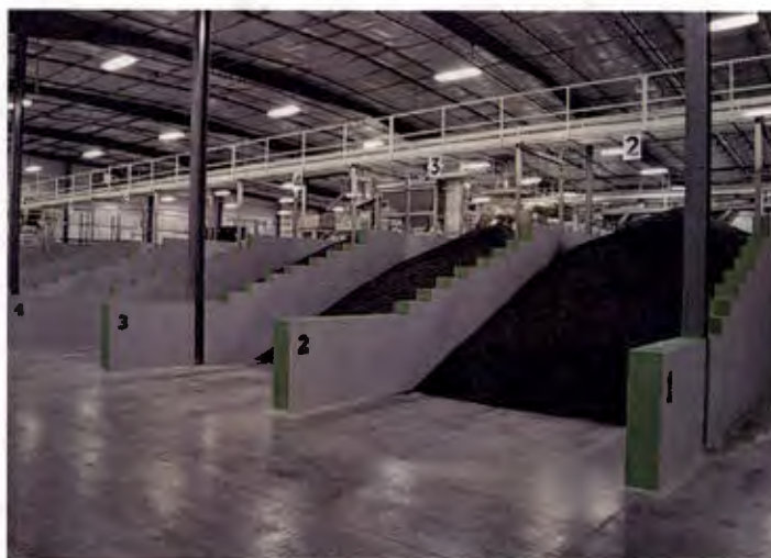
Here, large batches of the Florikan fertilizers await quality control testing before being bagged up and sold. The high-tech process to coat the fertilizer in a porous polymer to control how quickly the nutrients dissolve in water was perfected with help from NASA. Credits: NASA/SPINOFF
