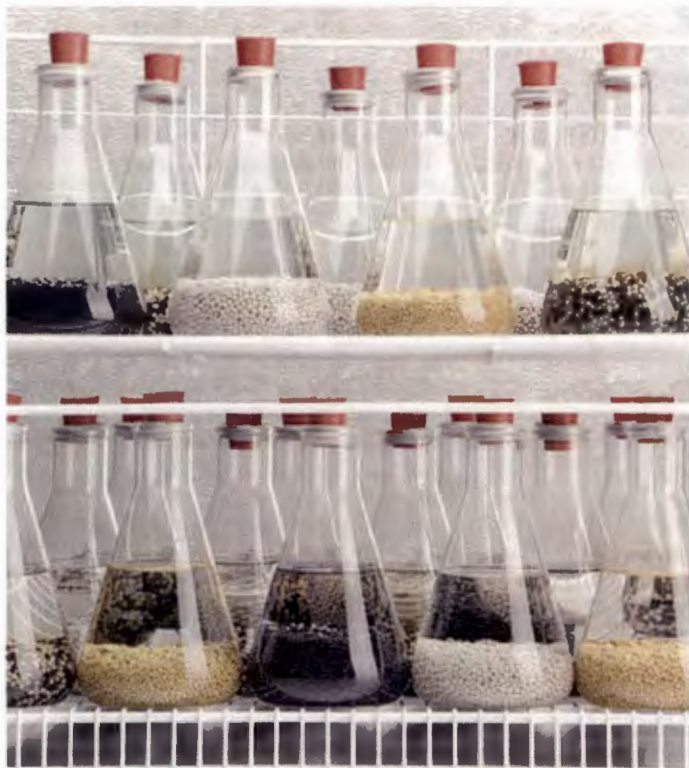
Every batch of Florikan coated fertilizer is tested to ensure the polymer coating allows the nutrients to dissolve at the expected rates. Small samples are placed in distilled water and held in an incubator at 100 °F for seven days. The quality control team checks the sample after one, three and seven days. Credits: NASA/SPINOFF
