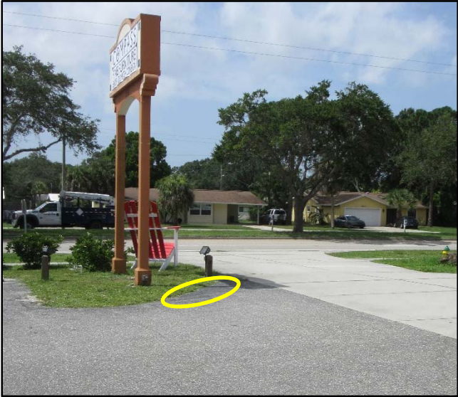
The yellow outlined area is where existing pavement is proposed to be removed to comply with the minimum five-foot setback from edge of pavement.
