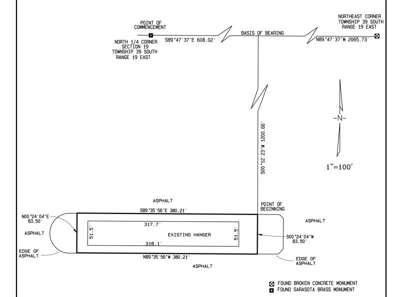
BEARINGS SHOWN HEREON ARE ASSUMED, AND REFER TO THE NORTH LINE OF THE NORTHEAST 1/4 OF SECTION 19, TOWNSHIP 39 SOUTH, RANGE 19 EAST BEARING BEING SOUTH 89'47'37" EAST, BETWEEN THE TWO MONUMENTS DEFINING SAID LINE, AS SHOWN HEREON.
