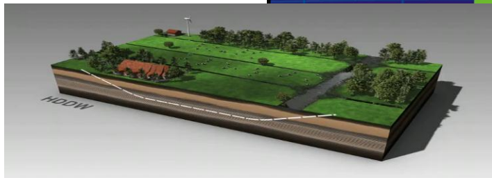
Horizontal Directional Drilled Wells
