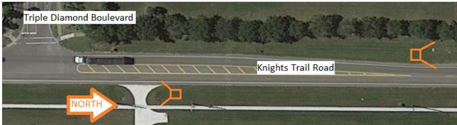
A speed trailer was placed on the East shoulder of Knights Trail Road facing northbound traffic. After at least a week of collecting data, the same speed trailer was moved to the west shoulder of Knights Trail Road facing southbound traffic.
