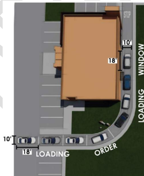
Figure 3.6.3. Stacking Requirements (Illustrative Purposes Only)
