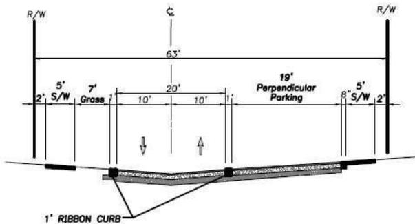
**INVERTED CROWN 63' RIGHT-OF-WAY SECTION**
