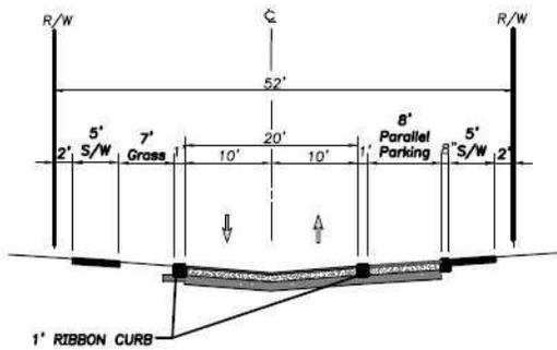
**INVERTED CROWN 52' RIGHT-OF-WAY SECTION**
