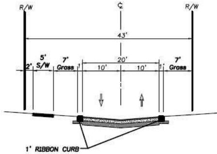
**INVERTED CROWN 43' RIGHT-OF-WAY SECTION**
