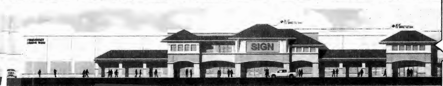
1 (JACARANDA BLVD.) GROCERY ELEVATION SIGNAGE REQUIREMENTS: 1.6 SQ. FT. PER LINEAR FOOT OF BUILDING FRONTAGE OR 150 SQ. FT. TOTAL, WHICHEVER IS LESS. ALLOWED: SIGN 150SF TOTAL SIGN PROVIDED: 119.06 SQFT PHARMACY PROVIDED 21.73 SQFT TOTAL 140.81 SQFT SIGNAGE SHOWN
