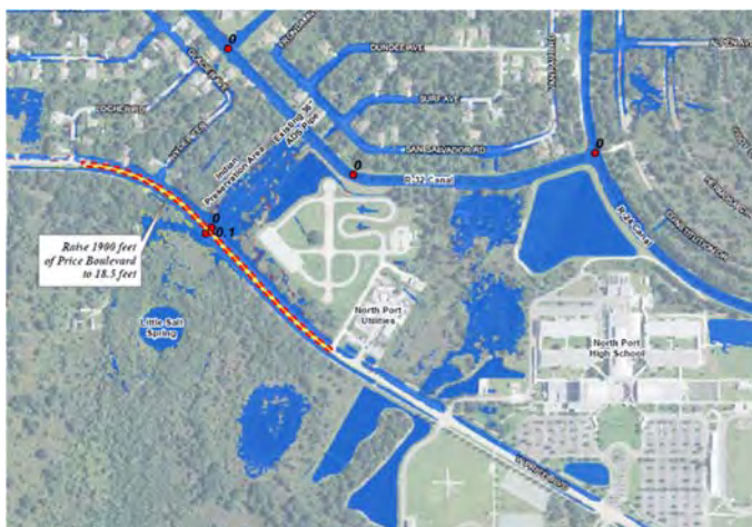
Raising of Road (as Conceived by Ardaman, 2014) and Barrier Wall (as illustrated by Crane Materials International, 2016)
