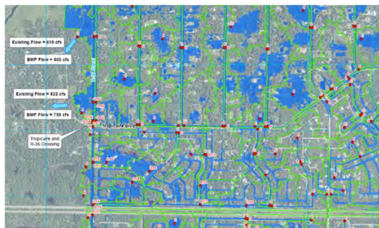
R-36 Canal Culvert Crossing Improvements Tropicaire (as Conceived by Ardaman, 2014)
