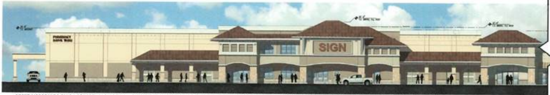
FRONT (JACARANDA BLVD.) GROCERY ELEVATION. SIGNAGE REQUIREMENTS: 1.5 SQ. FT. PER LINEAR FOOT OF BUILDING FRONTAGE OR 150 SQ. FT. TOTAL, WHICHEVER IS LESS. ALLOWED SIGN: 1500 SF TOTAL SIGN PROVIDED: 116.24 SQFT. PHARMACY PROVIDED: 27.73 SQFT. TOTAL: 143.97 SQFT. SIGNAGE SHOWN.
